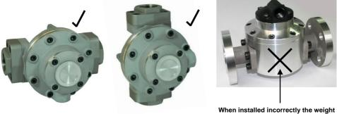
When installed incorrectly the weight of the rotors will bear down on the base of the measuring chamber.
