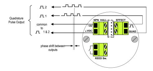
**2.3.6 Bi-directional flow** Combining the Quadrature feature and model PD2 pulse discriminator module produces forward & reverse outputs both of which may be integrated to provide a "net" reading. The RT12 flow rate totaliser will take both output & will perform the "net" flow function.
